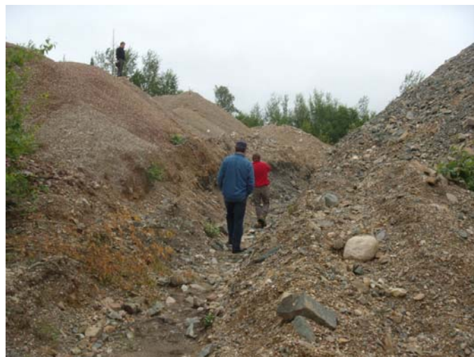
Figure 6. 14,000 tonne crushed ore stock pile on left, unknown quantity of un-crushed material on right.
