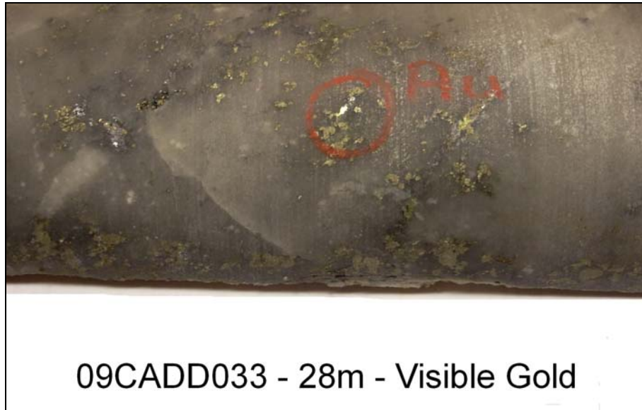
Figure 3. Visible gold in chalcedonic quartz vein material in association with galena and pyrite from 09CADD033 at 28m.
